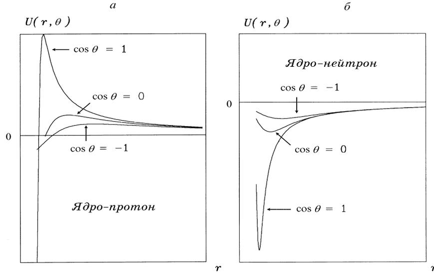
Figure 1: The drawings of potential energy dependence from spin orientation: *a* - potential energy of protons scattering on polarized target with  $r_e/r_N = -2$ ,  $r_N/r_s = 1,5$ ; *b* - the same for neutrons with  $r_e/r_N = 0$ ,  $r_N/r_s = 1,5$
